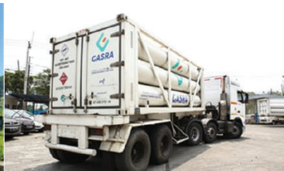
GTM Industri GTM : 20 Feet Capacity : 2.800 sm 3
