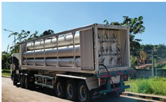
GTM Industri GTM : 40 Feet Capacity : 6.300 sm 3
